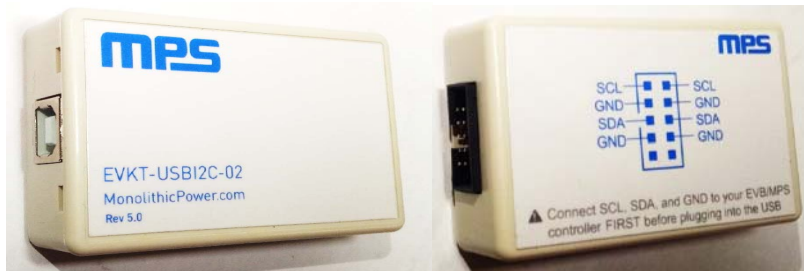
Figure 1: USB to I 2 C Communication Interface
