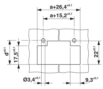
Dimension d depending on the wall thickness (W) in mm: W=1: d=21.4
