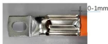
Figure 7: Crimp the ring tongue
