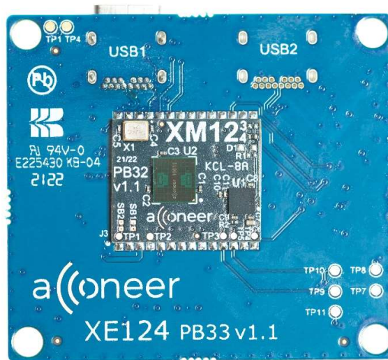
Picture 2. The XE124 top side where XM123 is mounted.
